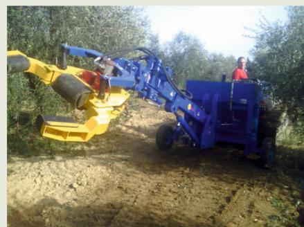
The MOR-001 is a reversed umbrella with lifting columns (for connection to dozer) that allow greater elevation for discharge on a trailer. The vibrating system that shakes the trunk is integrated in the umbrella. A hydraulic unit (max 30 hp) is connected to pdf tractor.
