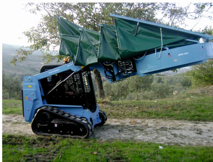
**MOR-003 model completes the range, a machine highly innovative: a hydrostatic machine multi-function (or skid loader) with standard attack for connecting of the reversed umbrella and head vibrating.**
